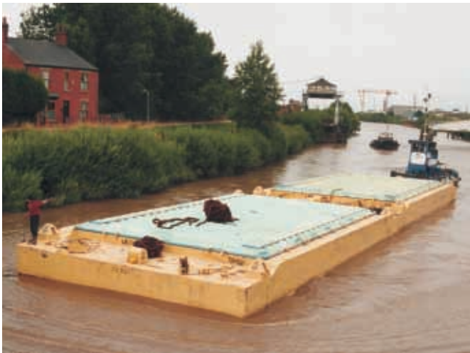
John Dean's pusher tug pushing two LASH (Lighter Aboard Ship) barges on the River Ouse at Selby in Yorkshire. Each LASH barge holds approximately 380 tonnes of rice, from the Mississippi region of the USA. A 'mother' ship loads a complement of LASH barges for the transatlantic voyage to Rotterdam where the feeder vessel Spruce takes on the LASH barges bound for the UK. Around 15 loaded barges are discharged in the Humber every seven to eight days at a jetty in Immingham. Barges are pushed in pairs to various moorings to await the trip to Selby. Westmill Foods mill in Selby has gradually increased the tonnage received by LASH barges, which are discharged by grab crane at a wharf immediately next to the mill. Approximately three full barges per week are handled in Selby removing the necessity for the equivalence of 95 lorry trips per week in and out of the mill. The mill is able to call up the barges to meet its requirements. The empty LASH barges are taken back down the Ouse and into the Humber, often loading steel from Corus in Scunthorpe for export to the USA. (Source: Mike Brown)
