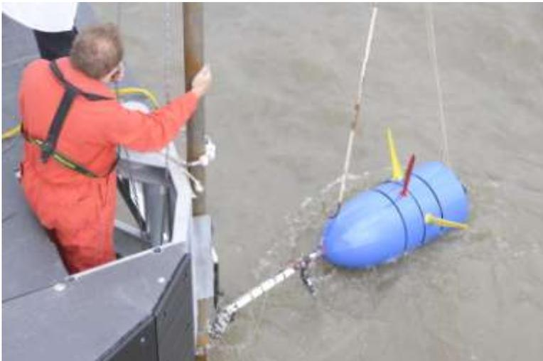
*A floating turbine is lowered into the Thames for trials to test how sustainable energy can be generated from tidal power*
